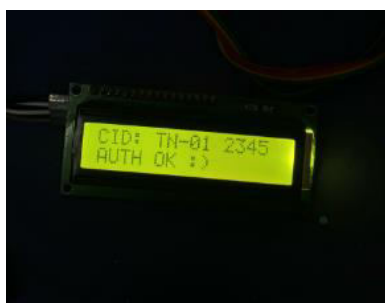
Figure 4.3: The output on display when vehicle check-in
